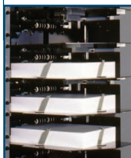
The 2.5" bin capacity conveniently loads 11 lb. to 12-pt. cover stock of paper sizes ranging from 4.72" x 5.52" to 14" x 20".
